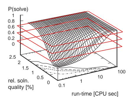
Typical SQT curves for SLS optimisation algorithms applied to instance of hard combinatorial optimisation problem:
