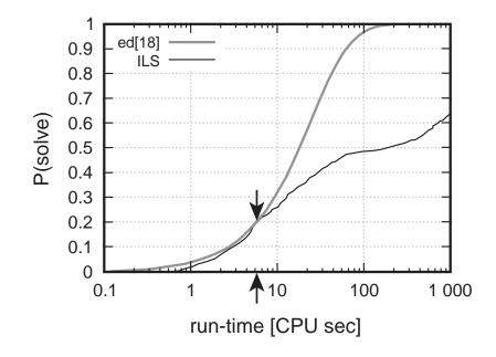
'ed[18]' is the CDF of an exponential distribution with median 18; the arrows mark the point at which stagnation behaviour becomes apparent.
