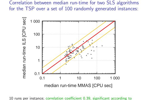
10 runs per instance; correlation coefficient 0.39, significant according to Spearman's rank order test at  $\alpha = 0.05$ ; p-value =  $9 \cdot 10^{-11}$ .
