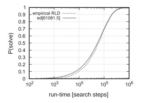
The optimal fit exponential distribution obtained from the Marquard-Levenberg algorithm passes the  $\chi^2$  goodness-of-fit test at  $\alpha = 0.05$ .
