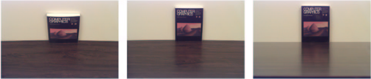
Figure 2: The table surface becomes more specular at grazing angles (image from [4], used without permission).
