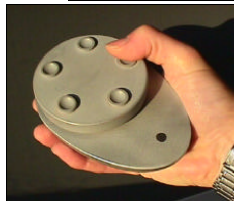
Figure 8: Representative integral-handle concept prototypes, exemplifying force-feedback wheels with a variety of Discrete Selector schemes. (a) Iconic spokes; (b) edge-buttons; (c) top-selectors. (b) and (c) selectors would be physically distinctive with the non-supporting hand like an old rotary phone
