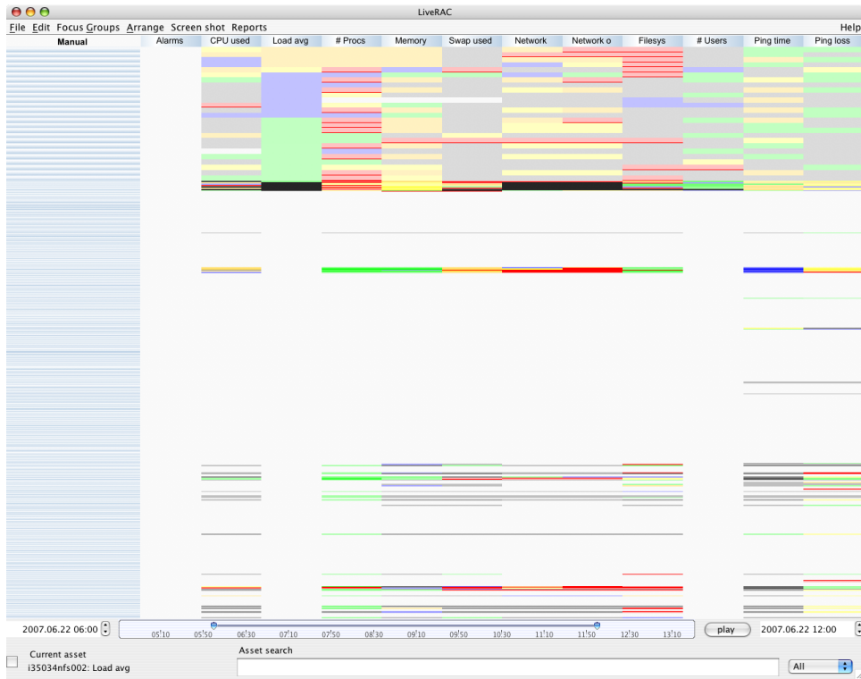
Figure 5. High used memory levels tripped the critical threshold values (red) for these two systems. Zooming in on the two flagged systems, the author discovered the SWIFT data collection system was returning erroneous negative memory values. This was reported to the data collection team, who were able to fix the problem the day before they received complaints from members of the network operations team that some of the systems were reporting strange memory values.
