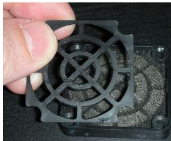
Figure 88 Removing the Filter Grille
