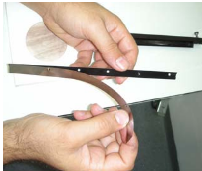
Figure 53 Removing the Roller Knife from the Knife Clamp
