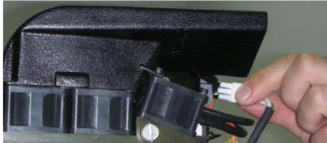
Figure 23 Disconnect Power Cable to UV Lamp
