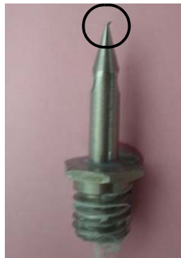
Figure 11 Magnification of a Bent Needle Tip (Example)
