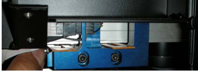
Figure 114 Orange Spacers between Encoder and Bracket.
