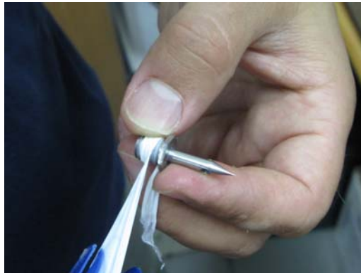
Figure 15 Wrapping Thread-Seal Tape
