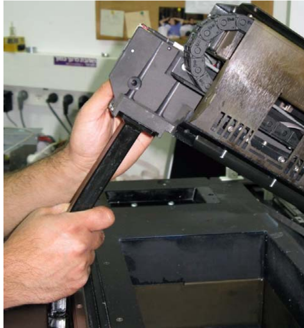
Figure 83 Lift Jig Under Y-axis Carriage
