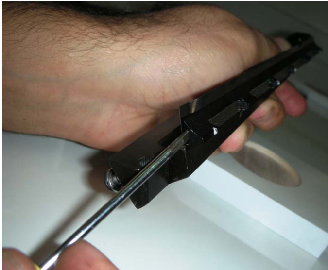
Figure 52 Prying Apart the Clamp from the Roller Waste Collector
