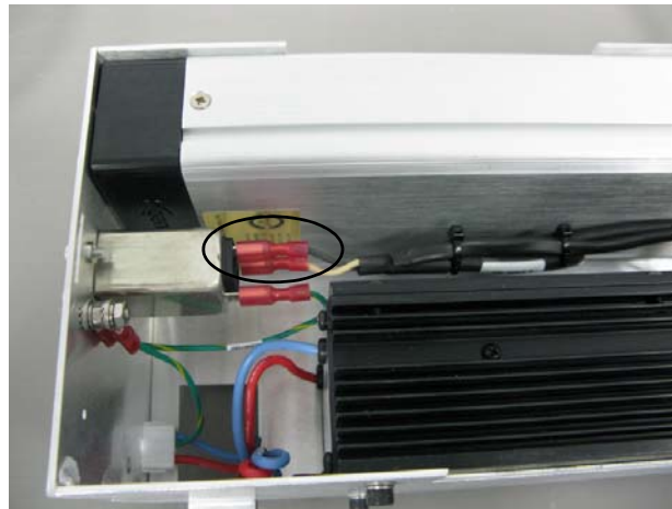
Figure 141 Wires Connected to the UV Power Socket
