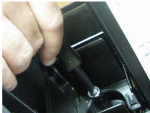
Figure 13 Removing Needle with Socket
