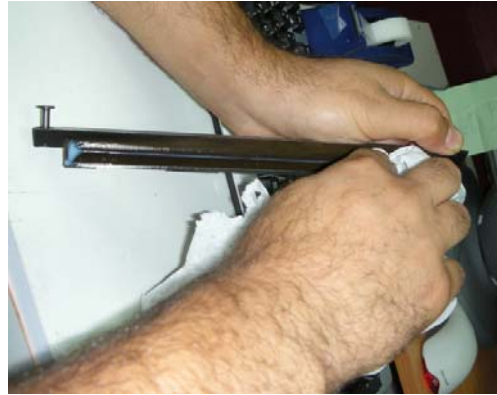
Figure 58 Roller Waste Collector Cleaning
