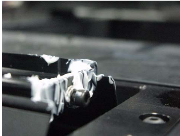
Figure 40 Wiper Waste Collector with Paste—Side View
