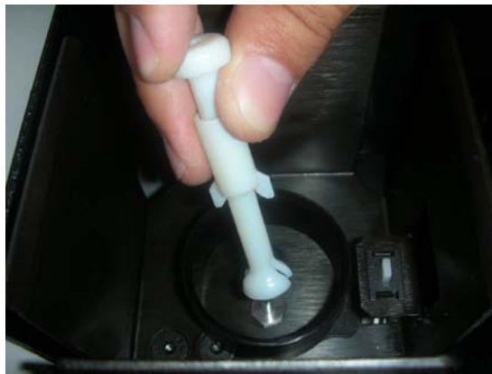
Figure 17 Placing a Dome on a Needle
