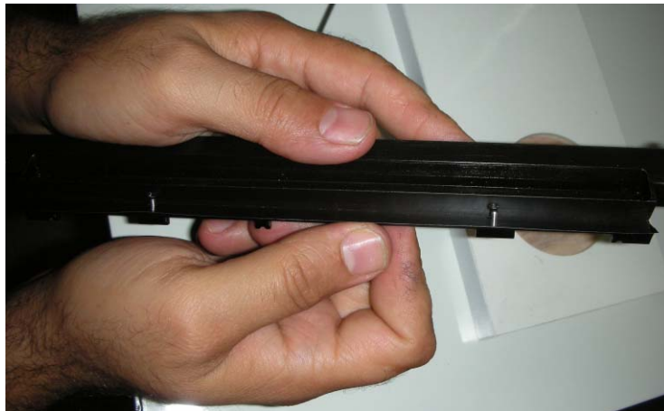
Figure 59 Align Roller Knife Clamp with the Roller Waste Collector
