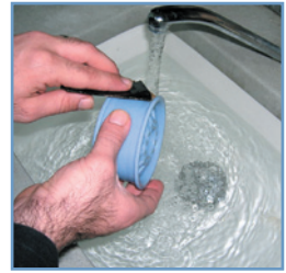
Figure 2. Wet-sanding. Wet-sand the model with 320-grid sandpaper.
