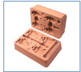
Picture 3. The sand casting mold – forming the cavity.
