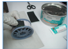
Figure 4. Dry sanding. Dry sand the model with 400-grit sandpaper.
