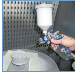
Figure 6. Apply Primer Paint.
