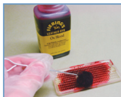
Figure 2. Apply aniline dye Aniline dye is applied to the model by brushing (shown), or dipping.
