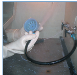
Figure 1. Removal of support material.
