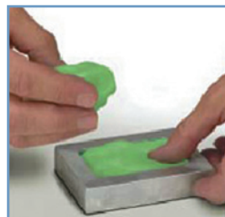
Figure 2. Placing the Objet model inside the mold.
