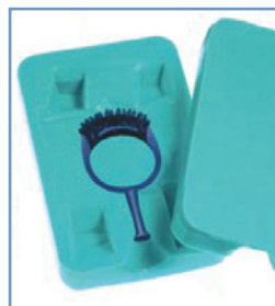
Figure 3. Finished mold can be complex, and even include spiral plugs.
