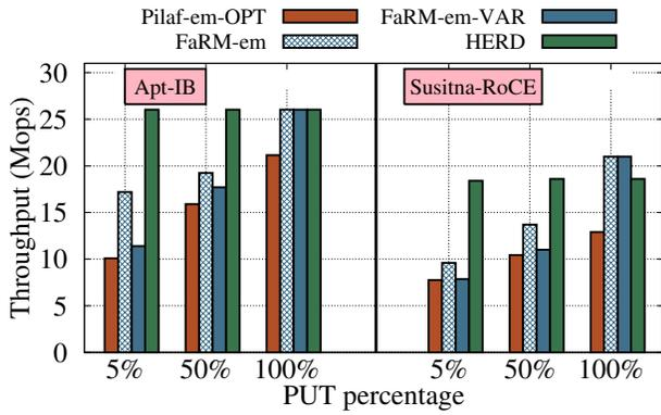
Figure 9: End-to-end throughput comparison for 48 byte key-value items
