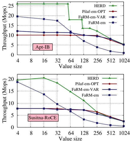
Figure 10: End-to-end throughput comparison with different value sizes
