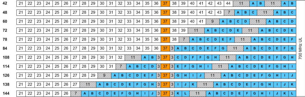
Figure 7: The FCC’s band plan for 600 MHz. Each row corresponds to a different clearing target and shows which channels would be repurposed and which would remain for TV broadcasting.
