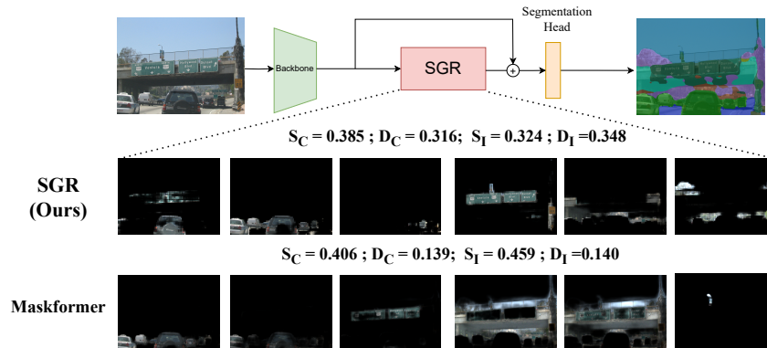
Figure 1. SGR learns to group pixels into latent tokens based on semantic similarity (top); the tokens are refined using a Transformer and back-projected to enhance the original features for segmentation. Notably, the resulting tokens are more semantic than prior work, as measured by the proposed class-semantic ( S_C ) and instance-semantic ( S_I ) metrics ( \downarrow is better), and are more diverse ( \uparrow is better), as measured by proposed diversity metric at class ( D_C ) and instance-level ( D_I ) (see Maskformer [19] in the bottom).
