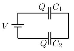
First we need to know how much charge is placed on the capacitors. Since they are in series they must both acquire the same charge, Q.
