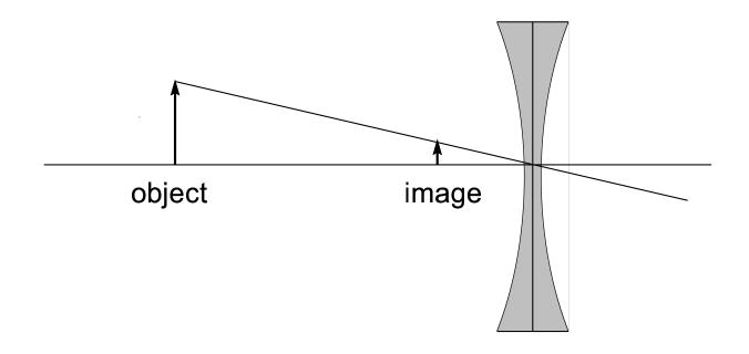
We can also calculate the focal length of the lens:
