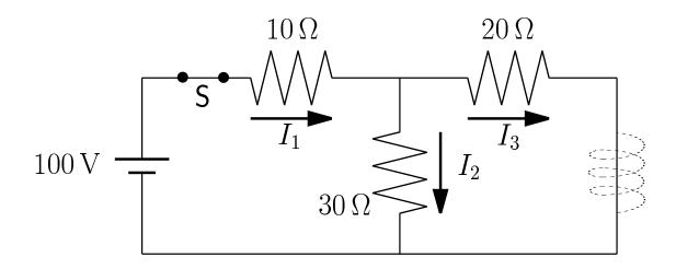
So the resistors  $R_2$  and  $R_3$  are in parallel with equivalent resistance
