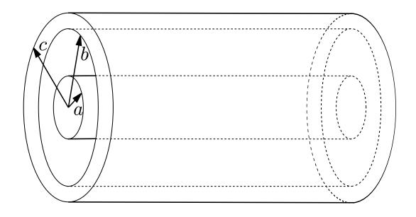
A very long, uniformly charged cylinder with volume charge density  $\rho$  and radius a is coaxial with a conducting cylindrical shell with inner radius b and outer radius c, as shown above. (a) Calculate and plot the electric field strength E as a function of radius r. (b) What is the surface charge density  $\sigma$  on the inner surface of the shell (r=b)?
