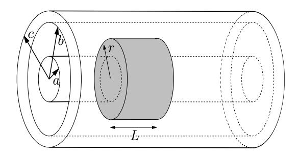
In this region, the Gaussian surface is in empty space, completely enclosing the charged cylinder. Therefore, the enclosed charge is constant
