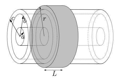
Now the Gaussian surface is outside of all the cylinders and, because the cylindrical shell has no charge, the enclosed charge is just given by Eq. (10) again.
