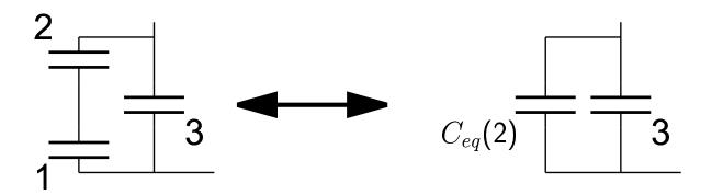
The first two capacitors can be represented as a single capacitor now, so this time we just have to calculate the equivalent capacitance of two capacitors in parallel
