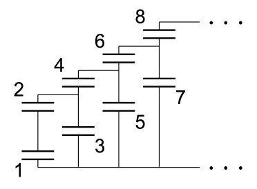
A group of identical  $C=1\,\mu\mathrm{F}$  capacitors are connected recursively, as shown above. Calculate the equivalent capacitance of (a) the first two capacitors, (b) the first three capacitors. (c) Repeat, up to the eighth capacitor. (d) (Optional.) In the limit of infinitely many capacitors, what is the equivalent capacitance of this configuration? (Hint:
