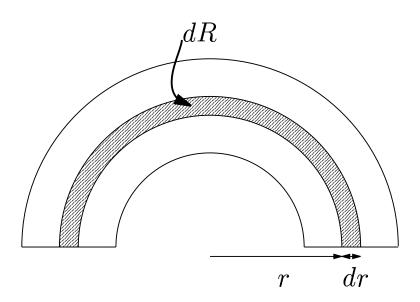
Now A on the inner surface of the section is  $\pi rt$  and on the outer surface of the section it is  $\pi(r+dr)t$  so, if we take infinitesimal sections  $dr\to 0$  then A is a constant for each section.
