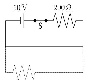
So the circuit just consists of a battery and a resistor, giving a current across the battery at time 0
