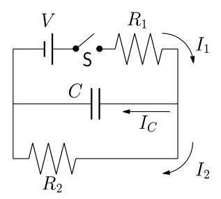
$I_C$  is just the rate charge passes through (or builds up on) the capacitor so
