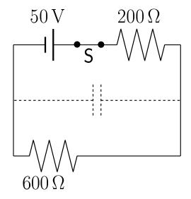
So we just have two resistors in series with a battery giving a current across the battery at time  $\infty$
