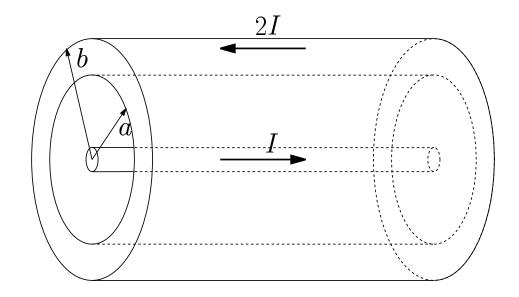
A very long coaxial cable consists of a thin inner wire and a concentric outer cylindrical shell with inner radius a and outer radius b. A current I runs down the inner wire and a current 2I comes back up the shell (uniformly distributed). Find the magnetic field  $\mathbf B$  at a distance r from the center for (a) r < a, (b) a < r < b, and (c) r > b. (d) Sketch a graph of B versus r.
