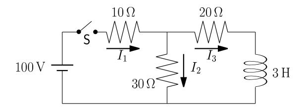
For the circuit shown above, find the currents  $I_1$ ,  $I_2$ , and  $I_3$  (a) immediately after switch S is closed and (b) a long time after switch S has been closed. After the switch has been closed for a long time, it is opened. Find the three currents (c) immediately after switch S is opened and (d) a long time after switch S was opened.
