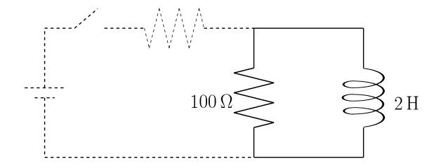
So, the time constant just depends on the inductor and the  $100\,\Omega$  resistor:
