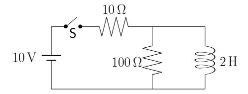
Given the circuit shown above, assume that switch S has been closed for a long time so that steady currents exist in the circuit and that the resistance of the inductor L may be considered to be zero. (a) Find the battery current, the current in the  $100\,\Omega$  resistor, and the current through the inductor. (b) Find the initial voltage across the inductor when switch S is opened. (c) Give the current in the inductor as a function of time measured from the instant of opening switch S.
