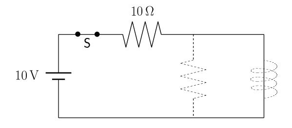
So the circuit just consists of a battery in series with a single resistor and the currents through the battery and the inductor are
