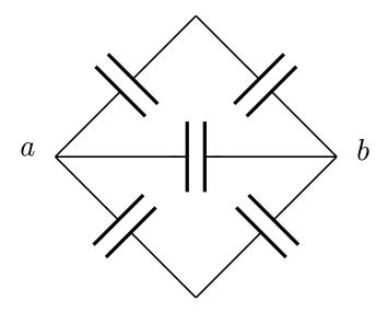
Five identical capacitors of capacitance  $C_0$  are connected in a bridge network as shown above. (a) What is the equivalent capacitance between points a and b? (b) Find the equivalent capacitance if the capacitance between a and b is changed to  $10C_0$ .
