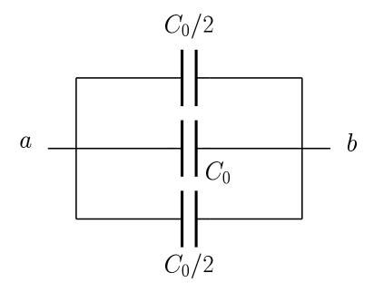
So the circuit is equivalent to the above diagram. Now we notice that we are just dealing with three capacitors, all in parallel so the equivalent capacitance is just
