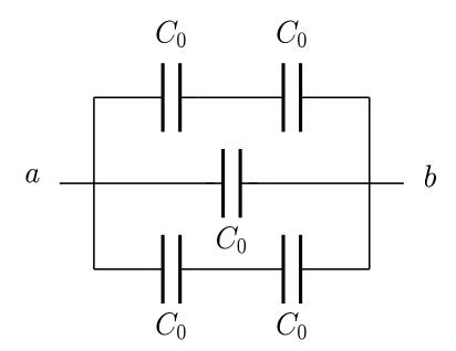
Now, we can't find any set of capacitors which are all parallel to each other but the top and bottom of the diagram each have two capacitors in series. The equivalent capacitance for each of these combinations is
