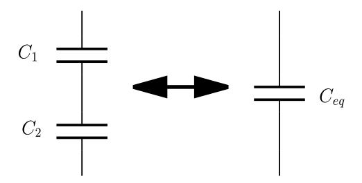
When two capacitors are connected in series, they are equivalent to of a single capacitor with capacitance
