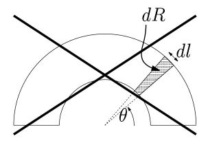
But it won't work! It fails because the length L=dl isn't a constant so you can't use  $dR=\rho\,dl/A$ . It is smaller at the inner radius than the outer.
