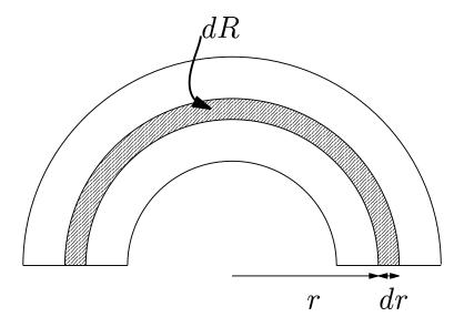
Now we are dealing with a bunch of pieces (resistors) which are side-by-side, or in parallel. So the equivalent resistance is given by
