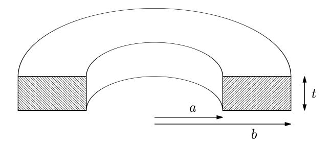
Find the resistance between the ends of the half ring shown above. The resistivity of the ring is  $\rho$ .
