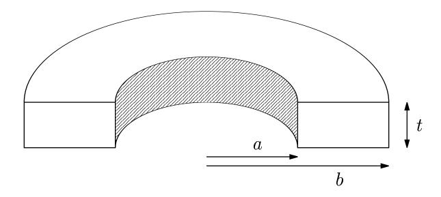
Find the resistance between the inner (shaded) and outer surfaces of the half ring shown above. The resistivity of the ring is  $\rho$ .
