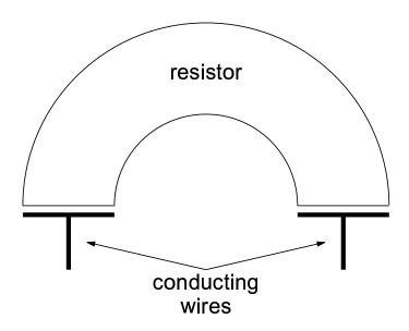
Schematically, we are trying to calculate the resistance of the resistor shown above.
