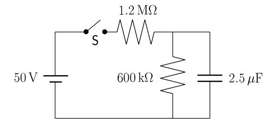
For the circuit above, (a) what is the initial battery current immediately after switch S is closed? (b) What is the battery current a long time after switch S is closed? (c) If the switch has been closed for a long time and is then opened, find the current through the  $600\,\mathrm{k}\Omega$  resistor as a function of time.
