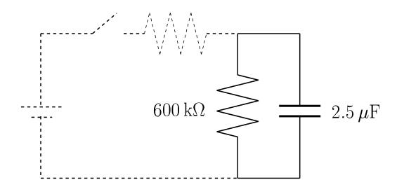
The capacitor starts with the final voltage it had when the switch was closed
