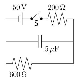
For the above circuit, (a) what is the initial battery current immediately after switch S is closed? (b) What is the battery current a long time after switch S is closed? (c) What is the current in the  $600\,\Omega$  resistor as a function of time?
